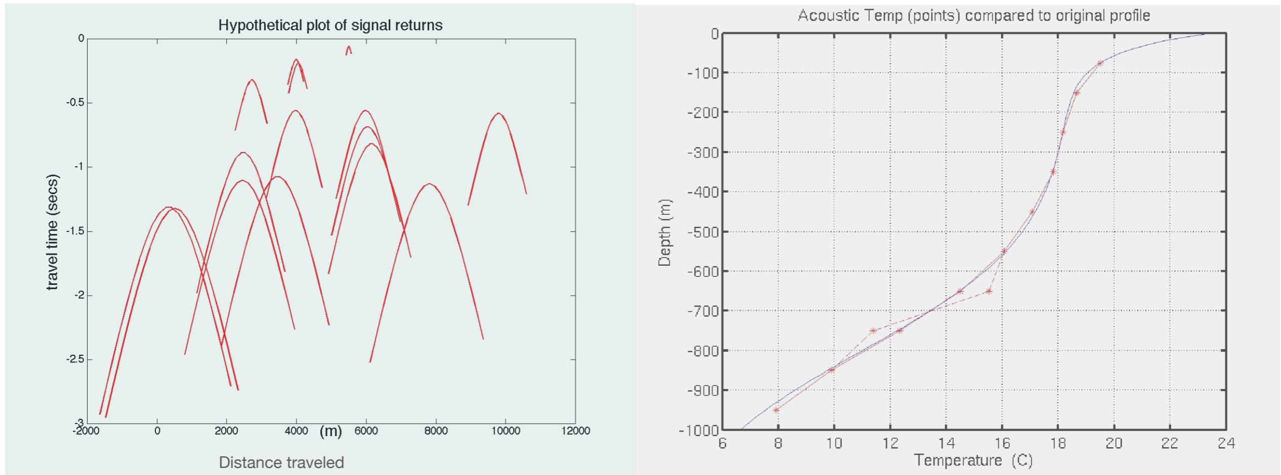
Left panel illustrates acoustic round-trip travel time to discrete backscatterers as a function of distance traveled by the ship. Note how the hyperbolae become broader with increasing depth. Right panel shows hypothetical reconstruction of temperature. The dashed line indicates error introduced due to errors in estimated speed of sound.
